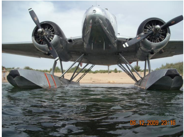
Twinbeech D18S on EDO/Bristol 7850 Floats. Two Pratt & Whitney Military R-985 450 hp 9 cylinder radial engines. Seating for pilots and 8 passengers.
