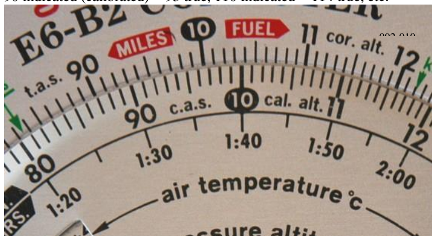
Figure 3b TAS at ~2700' Density Altitude — 90 indicated (calibrated) = 93 true, 110 indicated = 114 true, etc.
