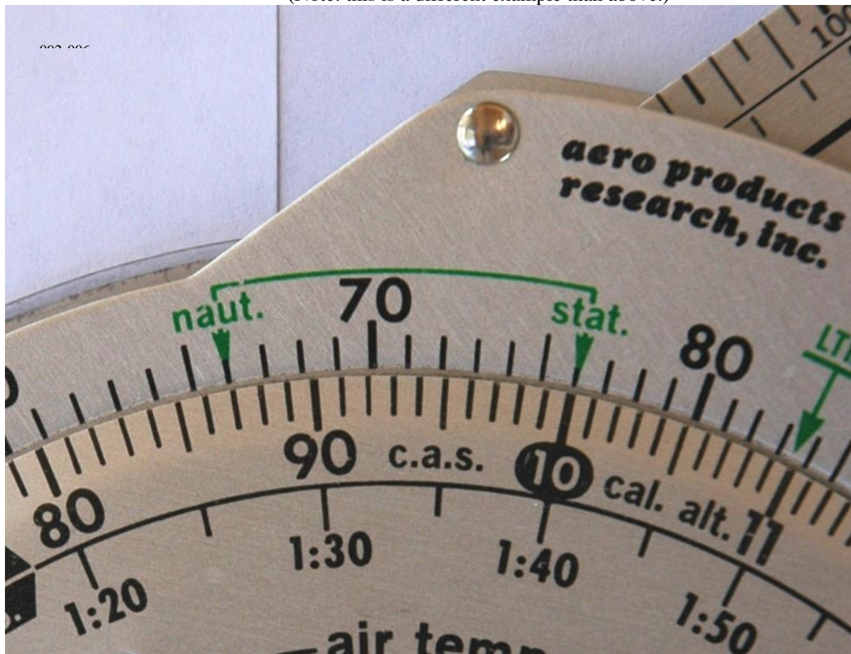
Figure 1 SM-NM Conversion —100 SM is 87 NM (Note: this is a different example than above.)
