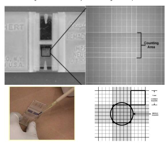
At the center of the chamber (there're actually 2 chambers on each hemocytometer) the etched lines form a 25 squares (5 squares by 5 squares) grid (Notice that there are 16 smaller squares etched into each of the 25 squares. These are a visual aid for counting cells). This is the area of the chamber that you want to use for counting. When a coverslip is placed on the hemocytometer, the dimensions of ALL 25 squares are:
