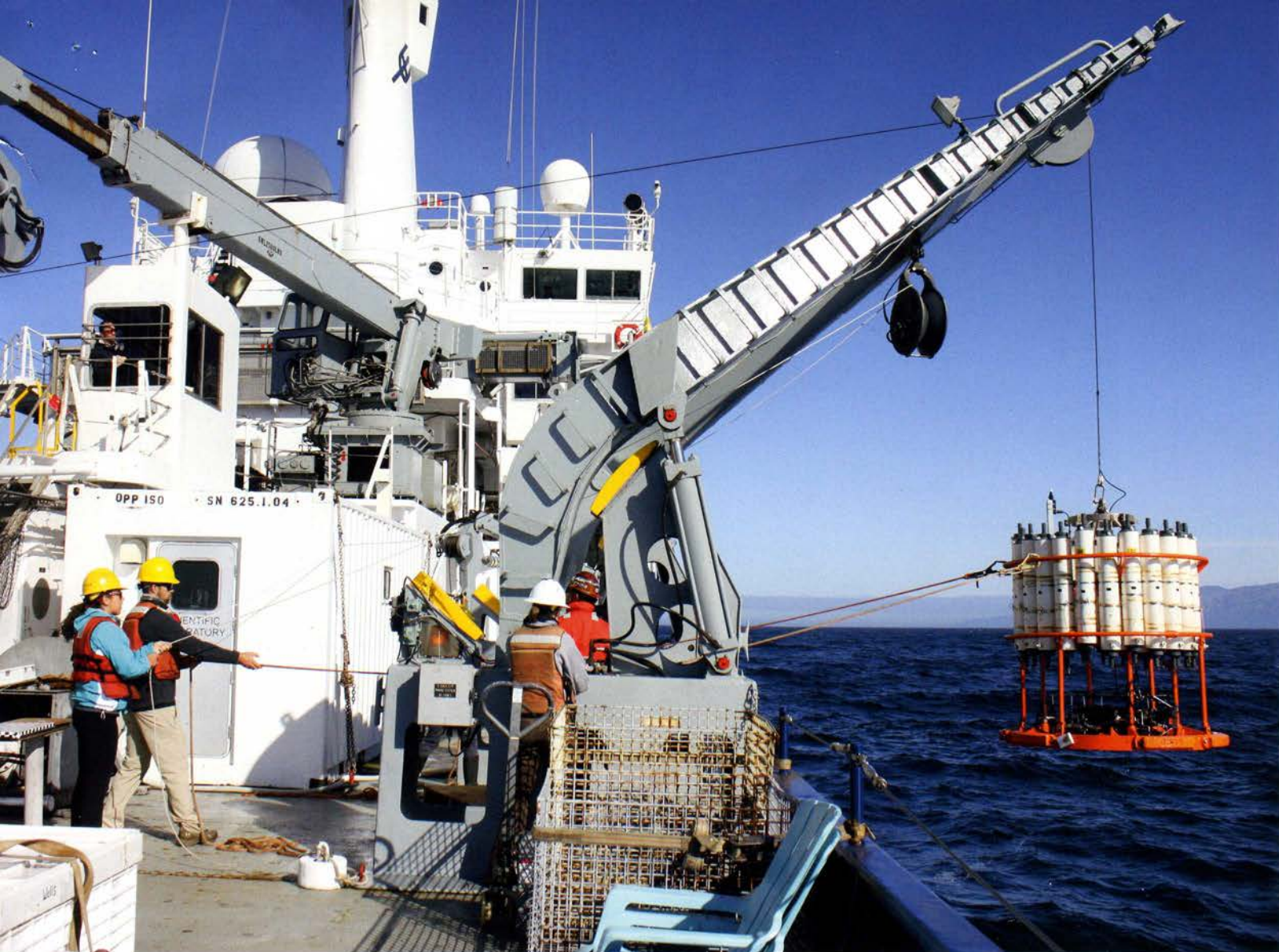
p. 36: Scripps Institution of Oceanography's resident technician preparing to launch a 20-liter Go-Flo bottle to collect trace-metal clean water samples for analysis aboard the R/V Melville during a research cruise from San Francisco to Seattle led by Dr. Cochlan.
