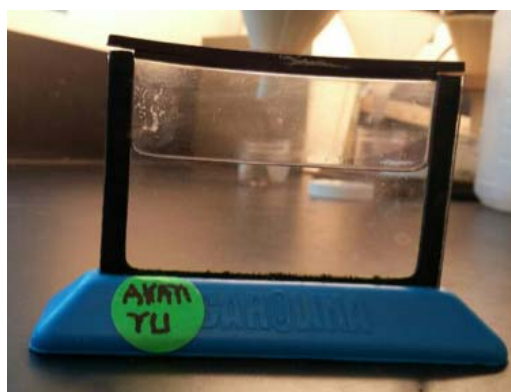
Figure 2: The microaquarium is 75 × 50 × 4-mm and holds about 5 ml
