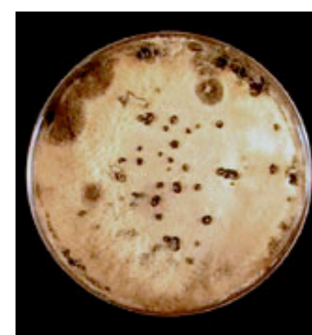
b. Stachybotrys cultured from 1m 3 of air outside Bldg 5. The normal habitat of Stachybotrys is soil. Soil excavation may have released spores into the air on this sampling day.
