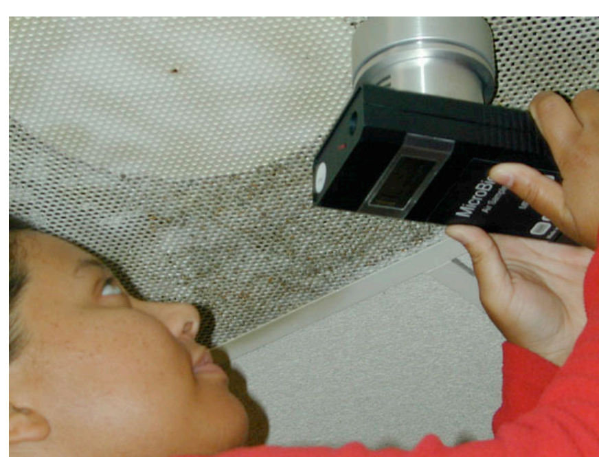
Figure 1. Air samples were collected with the MB2, which collects airborne bacteria and fungal spores from air flowing at 100 liters/minute through a series of 1 mm diameter air inlets, onto an agar filled 47 mm contact plate.
