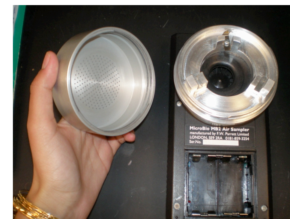
Figure 2. The MicroBio impact air sampler. Air is brought in so that airborne microbes are deposited on the surface of an agar plate.
