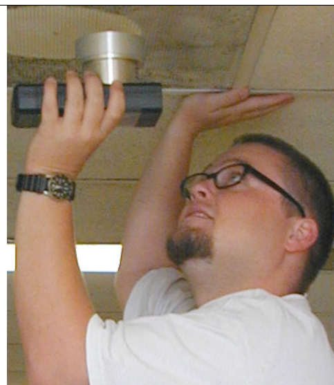
b) Collecting from a ventilation inflow.
