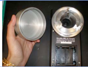
Figure 2. The Microbio impact air sampler. Air is brought in so that airborne microbes are deposited on the surface of an agar plate.
