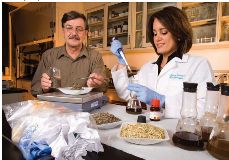
For ethanol research, technician David Bozzi weighs pulp recovered from garbage (a sample of which is in the plastic bag, at left) while microbiologist Diana Franqui adds glucose-releasing enzymes to a blend of plant material and pulp suspended in water. On the table, the plastic tray at left contains pulp from garbage; the tray at right holds rice straw—a plant waste left after rice harvest.
