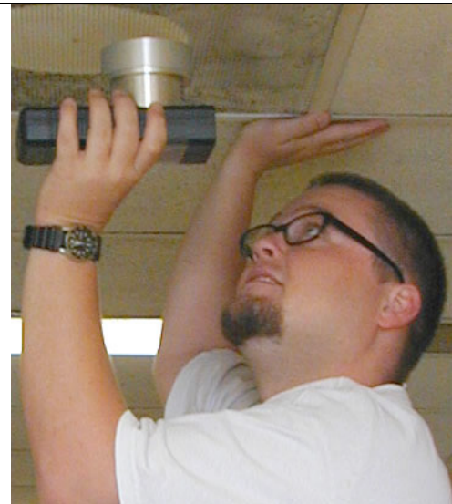
b) Collecting from a ventilation inflow.
